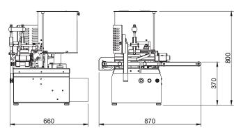
Automatic hamburger former machine with hopper with capacity for 20 Kg of mixture.
