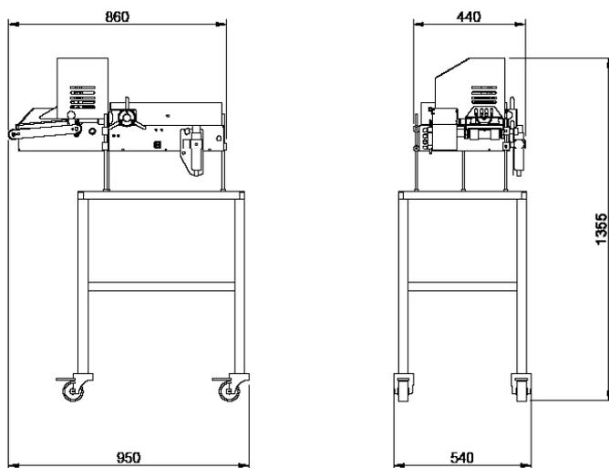
Automatic croquette and meatball former machine that may be coupled to any filler with simple or double product output and may also be connected to a batter & breading machine.
