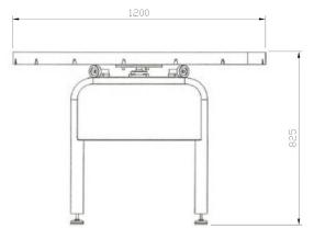
Rotary table to facilitate collection after exiting the breading machine or the frying line.
