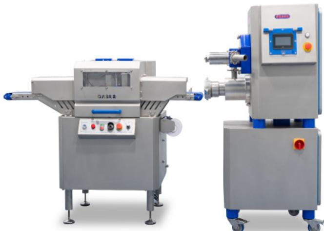
Production line for fixed weight portions for all types of product: grinded (free-flow), tablets, cylinders (cevapcici) and other shapes. Line consisting of a filler, mincer head and automatic portioner.
