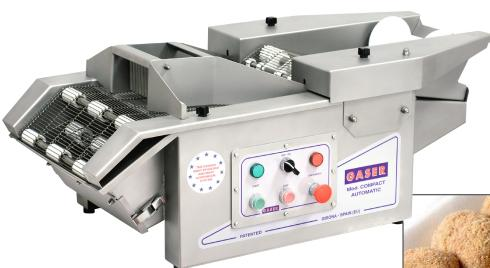
Compact model, a tabletop machine for small productions; specifically indicated for meatball and croquette manufacturing, as well as other similar products of small size.
