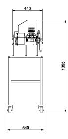
Automatic croquette and meatball former machine that may be coupled to any filler with simple or double product output and may also be connected to a batter & breading machine.
